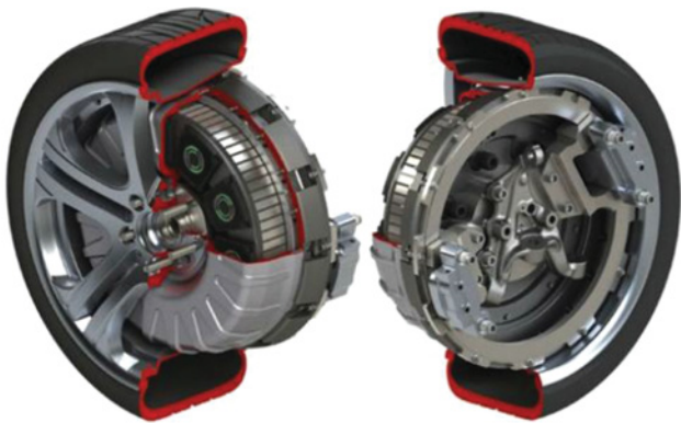
Figure 4.6 In-wheel electric motor, air cooled and axle water jacket [66]. Reproduced with permission of Protean Electric Ltd.
