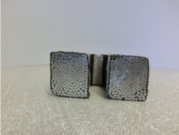
Figure 4.1 Pressed coil for high slot fill factor.
